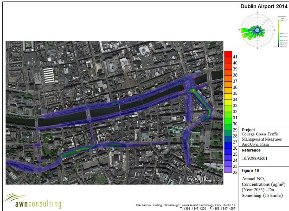
Figure 7.19 - Annual Mean Modelled NO 2 Concentration (µg/m 3 ) (Year 2035) (EFT Version 7.0) – Do Something Scenario
