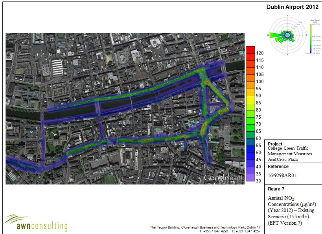
Figure 7.7 - Annual Mean Modelled NO 2 Concentration (µg/m 3 ) (Year 2012) (EFT Version 7.0)
